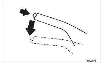
When parking on a hill, it is important to set the parking brake before placing the gear selector in Park, otherwise the load on the transmission locking mechanism may make it difficult to move the selector out of Park. As an added precaution, turn the front wheels toward the curb on a downhill grade and away from the curb on a uphill grade.
